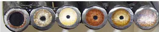
Build-up begins Combined build-up Chemical build-ups Hard water build-up Lime & calcium build-ups Plugged by ALL
